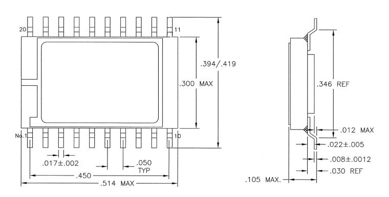
Note: Package and lid are electrically isolated from signal pads.
